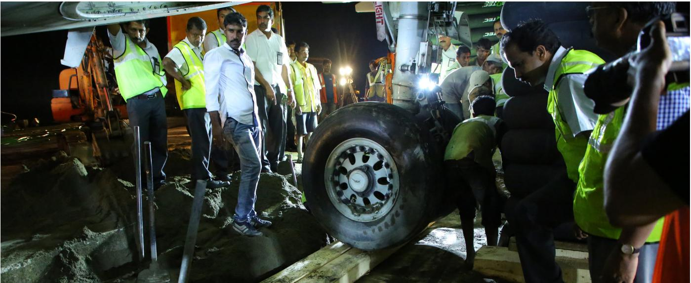
capable to recover narrow body aircraft like B737, B727, A319, A320, A321 etc or wide bodied aircraft in case of partial under carriage failure. CIAL's DART can also render its service to other airports, when needed.
